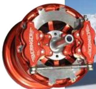
Dual braking system for tires over 29"
