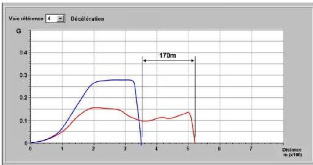
Nota: BERINGER brake pads used in the ALIR system have a friction coefficient that increases with the temperature allowing an increase of the deceleration when the lift decreases on the wings.
