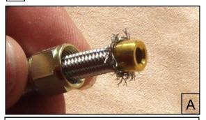
Push the olive onto the end of PTFE inner tube and under the stainless steel braid.
