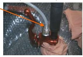
Open the bleeding screw of the caliper.
