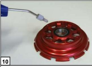
Clean with pressurized air or dry cloth the other wheel flange. Check that there is no dirt in the ring groove.
