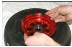
Pull up delicately by hand the side of the wheel with disc brackets.
