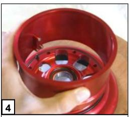
Place the wheel spacer on the wheel flange and press by hand, as shown above. Check that the 2 parts are in contact.
