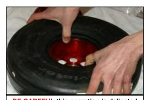
**BE CAREFUL this operation is delicate!**Pull up the tyre and push the wheel at the same time with the thumbs.
