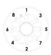
**BE CAREFUL**Respect the order when you torque tighten the 8 x M6 screws.
