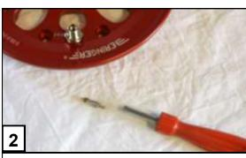
Remove the needle valve with the appropriate tool as detailed above.
