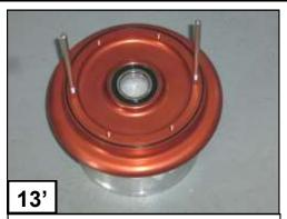
Place the 2 guide screws in 2 opposite holes on the wheel flange as illustrated above.
